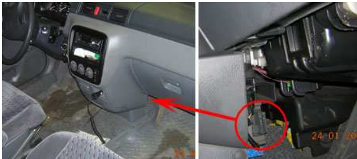
Behind Ashtray Typical Location For: 95-97 Accord (V6) 96-97 Accord (L4)
